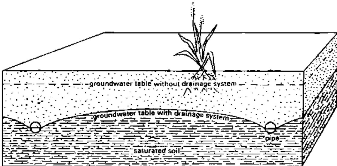
Figure 4. Pipe drains
